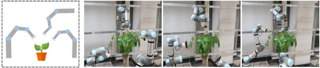
Fig. 2 Construction of a model of a plant using three robotic arms equipped with sensors. Reproduced with permission from Ref. [17], © IEEE 2019.
