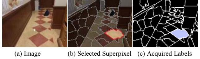
Figure 6: Label acquisition. We ask the oracle to label only the superpixels selected by our method (marked red in (b)). The remaining superpixels of the ground-truth map, shown in black in (c), are marked with the ignore label.
