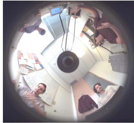
Figure 2. An example image captured by the omni-directional camera (shrunk to fit the page). While the captured image is warped, since the geometry of the mirror can be calibrated, it can be un-warped by the computer vision techniques.
