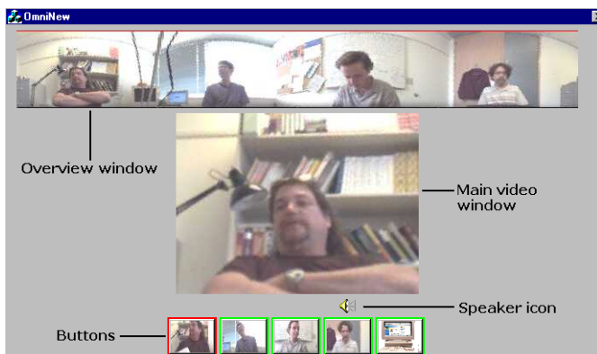
Figure 5: The user-controlled + overview interface. The window at the top is a 360-degree panoramic overview of the meeting room. The five buttons at the bottom are static images. Pressing these buttons changes the direction of the virtual camera. Pressing the fifth button gives control of the camera to the computer. The speaker icon above the buttons indicates who is currently talking.
