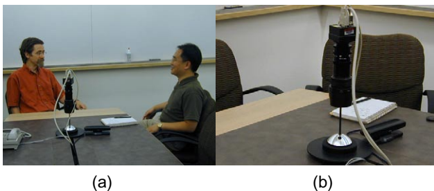
Figure 1. The omni-directional camera meeting capture environment. (a) People seated around the meeting table. (b) Close-up of the parabolic mirror and camera.
