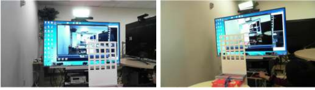
Fig. 12. An auxiliary pattern and an external camera is used to help calibrate the relationship between the camera rig, the screen, and the table top.
