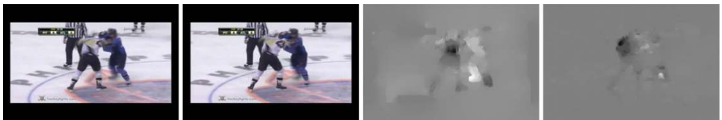
Fig 2. An example of optical flow images. Two consecutive frames, flow_x and flow_y , of the latter frame.
