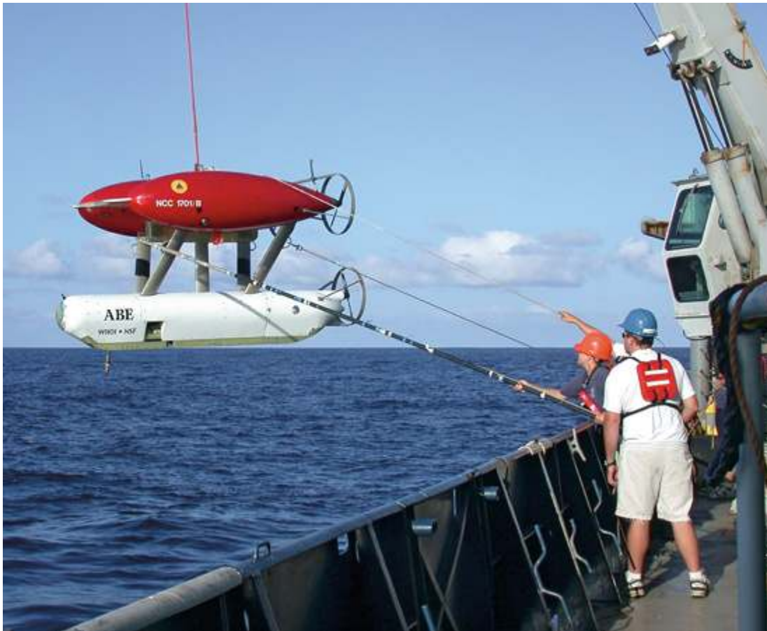
Figure 32: The Autonomous Benthic Explorer. (Dana Yoerger) [29]
