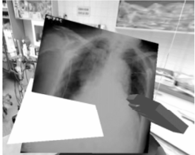
Figure 4. The user can grab document from VE and “bind” it into the virtual notepad by intersecting virtual notepad with the document and pressing a button.
