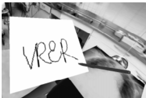
Figure 2. The virtual notepad is spatially registered with the physical tablet. When the user draws on the physical tablet, the virtual pen "draws" on the virtual notepad.
