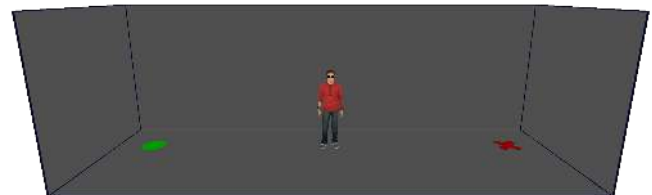
Figure 2: Layout of the experiment considering the physical boundaries of the IVE. The green dot represents the starting point and the red cross the end point of the path. The obstacle was placed in the middle of the working space, at 1m from the front screen and at 2m of the missing wall.
