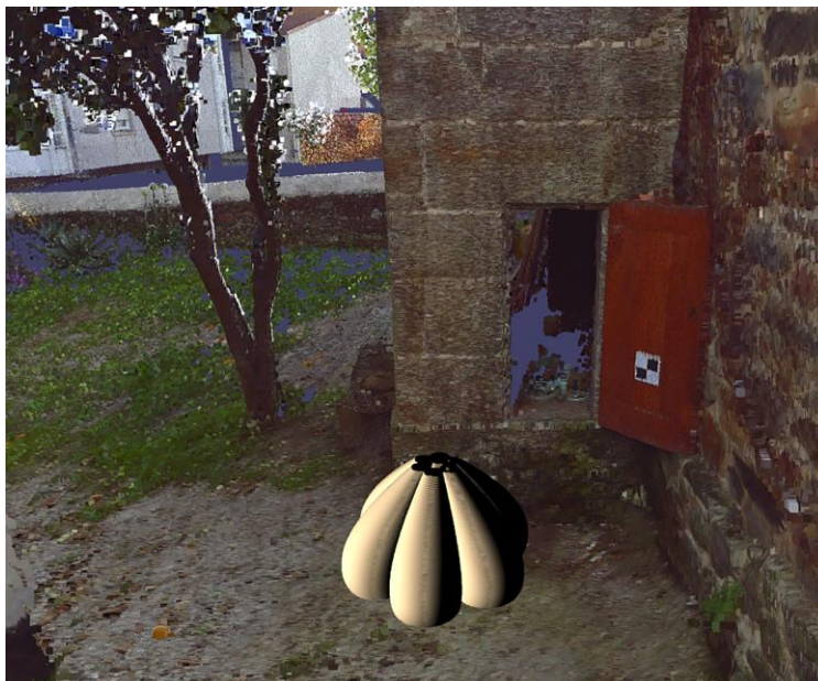
Figure 7. Shape designed in McNeel Rhinoceros and integrated in a real environment with our point cloud software.
