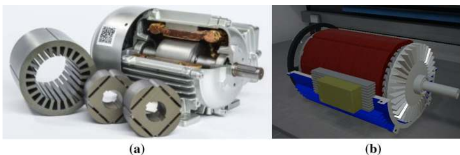
Fig. 3 Permanent magnet synchronous motor (PMSM) a authentic machine b 3D model in VR
