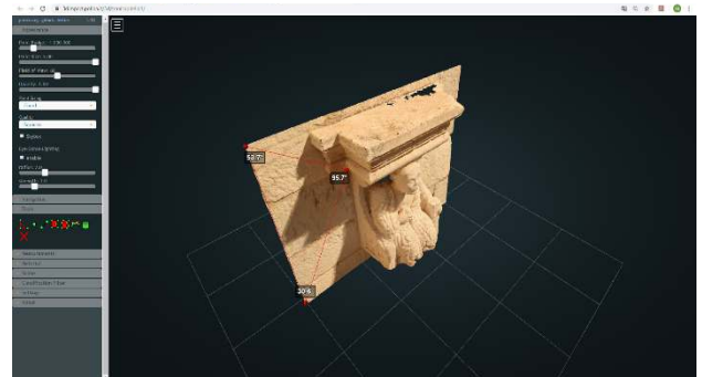
Figure 14. Screenshot, from active “3D” hotspot, showing point clouds of a capital in a web viewer.
