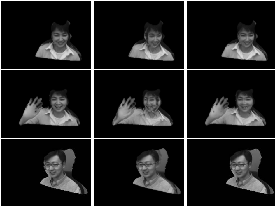
Figure 13: Comparison. In this figure we compare our results with two different approaches. Left column shows our results, in the middle column we display the results when the depth camera's depth estimate is directly used to render the virtual view and in the right column, we show the results of our algorithm but with pixel differencing as a dissimilarity measure. Direct rendering results in artifacts caused by registration errors and misalignments. Using pixel differencing, on the other hand, sometimes results in good renderings ( third row ) whereas in other cases it causes artifacts ( first and second rows ).
