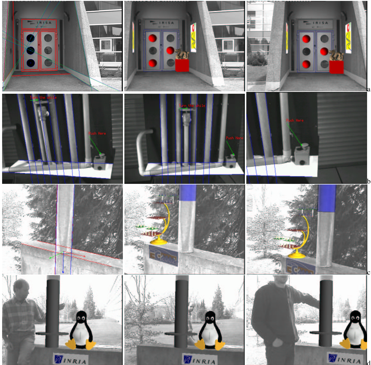
Figure 3: Pose computation and augmented reality in real environment without any landmarks. Since reliable points features are difficult to track in real environment, it is often useful to consider various features such as circles, lines or cylinder. In these experiments features are tracked using the moving edges algorithm in less than 5 ms. The whole process, tracking, pose computation, and rendering is achieved in real-time (i.e., 25Hz). In (a) circles and lines are considered in while in (b), (c) and (d) cylinders and lines are used. Figures (d) illustrates various cases of partial occlusions. This illustrates the versatility of the virtual visual servoing process wrt. the choice of the features extracted from the image.
