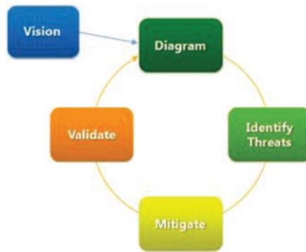
Fig. 9. Primary steps in the process of threat modeling [Microsoft 2010].
