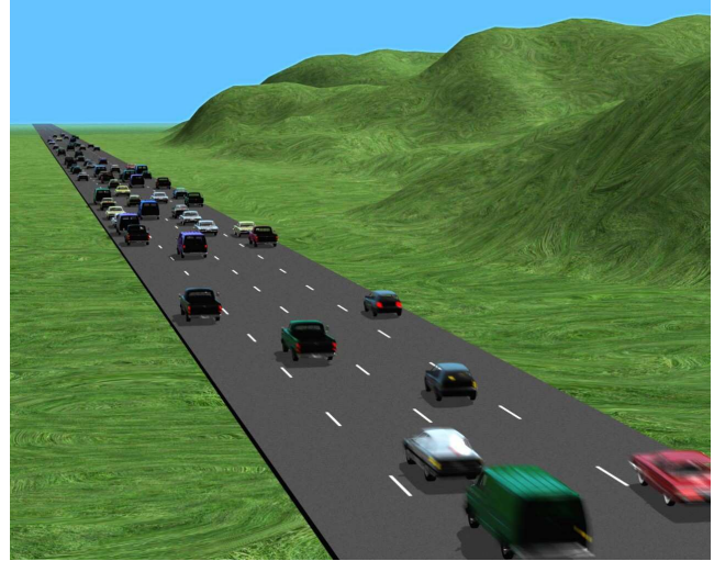
Figure 8: Images from our traffic jam scenario ( L = \{400m, 200m, 400m\}, N = 4, \rho = 1/2 ). The traffic of three consecutive stretches of a highway are reconstructed independently, and afterwards concatenated in a single visualization. In order to simulate a traffic jam, we generated the data such that the average velocity in the middle section was much less than in the other two.
