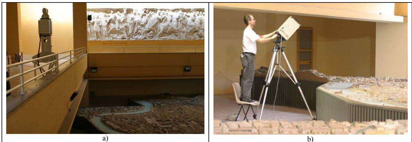
Figure 1: Equipment employed for the model of ancient Rome (“Plastico di Roma antica”): a) Laser Radar LR2000 by Leica MetricVision for long range; b) Vivid 910 by Konica-Minolta, a triangulation-based laser scanner, for close-ups
