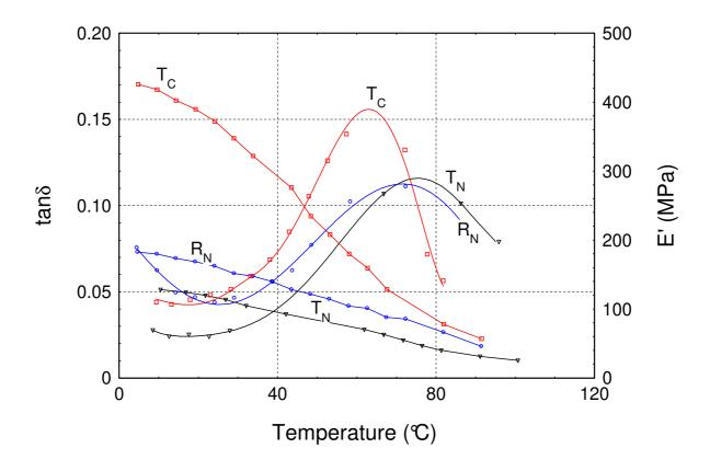
Figure 5: Evolution of the storage modulus and the loss factor versus temperature of normal wood and compression wood of Spruce (frequency: 5 mHz)
