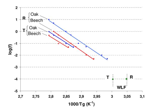
Figure 8: Arrhenius plot for beech and oak wood in radial and tangential directions
