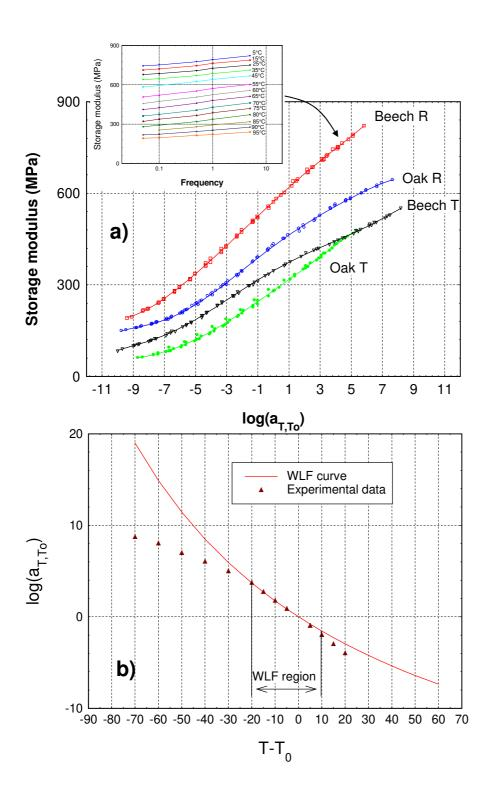
Figure 7 -a: Master curves for beech and oak wood in radial and tangential directions. b – The shift factor versus the temperature T-T<sub>0</sub> for the master curve of beech in radial direction. (Temperature of reference: 75°C).
