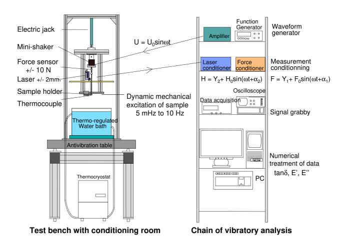
Figure 1: Schematic representation of the experimental device used: the  $\mathbf{WAVE}^\mathsf{T}$
