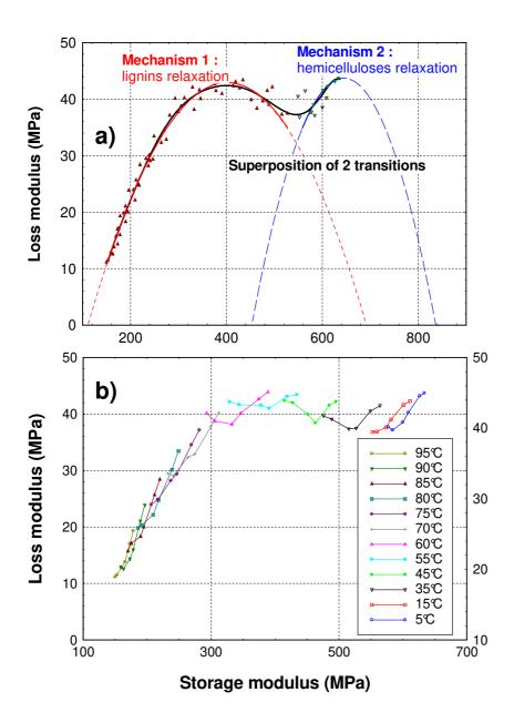
Figure 9- a : Cole-Cole plot for oak in radial direction. Measurements were carried out in the frequency range of  $5.10^{-3}$  Hz to 1 Hz and for temperatures between 5 and 95°C. b – Same experimental data t han in graph a, plotted according to the temperature.
