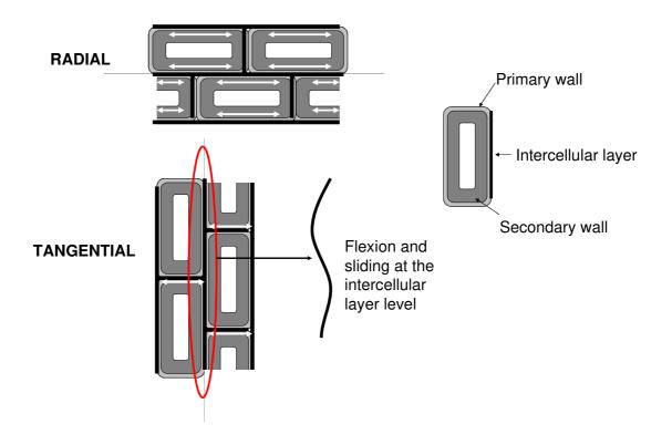
Figure 6: Schematic representation of softwood anatomical organisation in radial and tangential direction.
