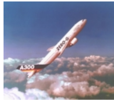
FIG. 2: Parabolic maneuver of the airbus A300 Zero-G.
