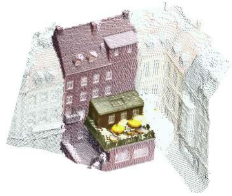
Fig. 15. Illustration of foveated depth inference with our proposed method. Different point density levels are denoted by different colors: Gray for sparsest, Brown for intermediate, Green for densest.
