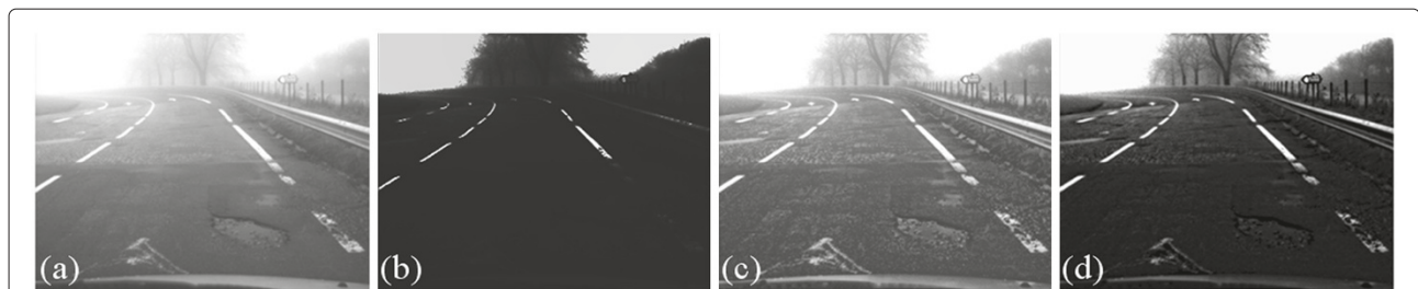
Figure 1 Visual comparison of the dehazing results of these methods for a misty gray image. These methods are [20,21] and the proposed algorithm using image filtering approach. (a) Original image, (b) [20], (c) [21], (d) the proposed algorithm.
