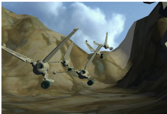
Figure 19: Scene from canyon flyby: computed using image compositing of sorted layers with 14 \times 14 terrain split. The highlighted terrain portion is one involved in a detected occlusion cycle with the ship above it, with respect to the bounding convex hulls.
