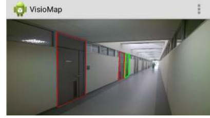
Fig. 8. A feedback on Google Glass display. We mark the rectilinear structures detected in the current scene with red and green colors, while the green frame can be employed to guide the users to proceed.
