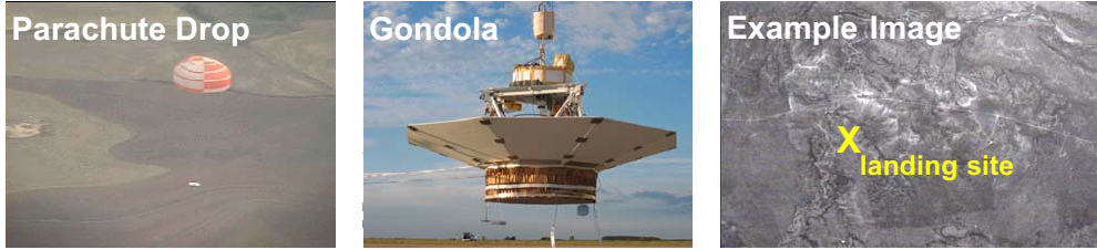
Figure 3: Pin-Point Landing Experiment on the NASA MSL Subsonic Parachute Drop Test (PDT). The gondola (center) was attached to a balloon that carried it to approximately 36 km altitude and then released it for descent on a parachute (left). During the descent, a nadir-pointing camera recorded images of the landing site (right), and an IMU provided measurements of acceleration and rotational velocity.
