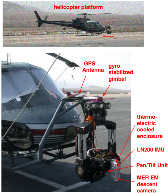
Figure 8: The sensor payload used for the DIMES field testing.
