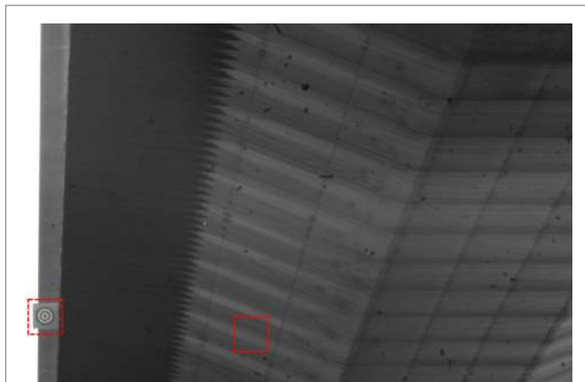
FIGURE 3 | Captured frame from DMS video records with marked custom-made target and natural feature target.
