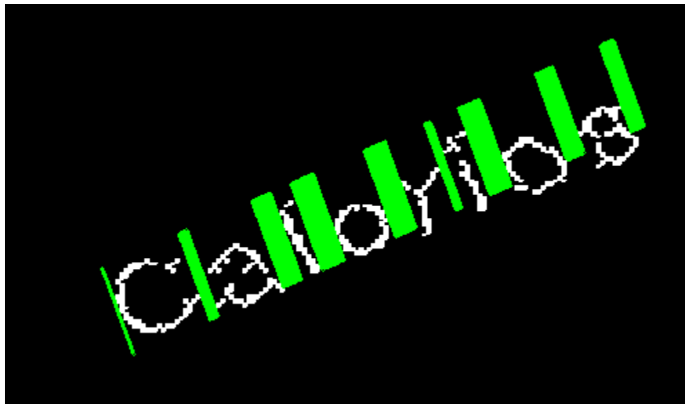
Figure 5.8 Gap identification from angular projections
