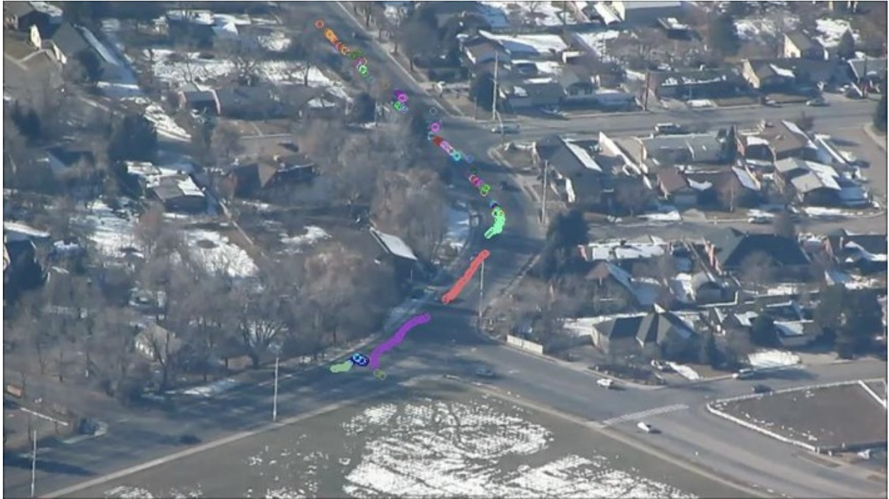
Figure 7.3: The GM-PHD tracks associated with one of the cars from the annotated section of the vehicle video.
