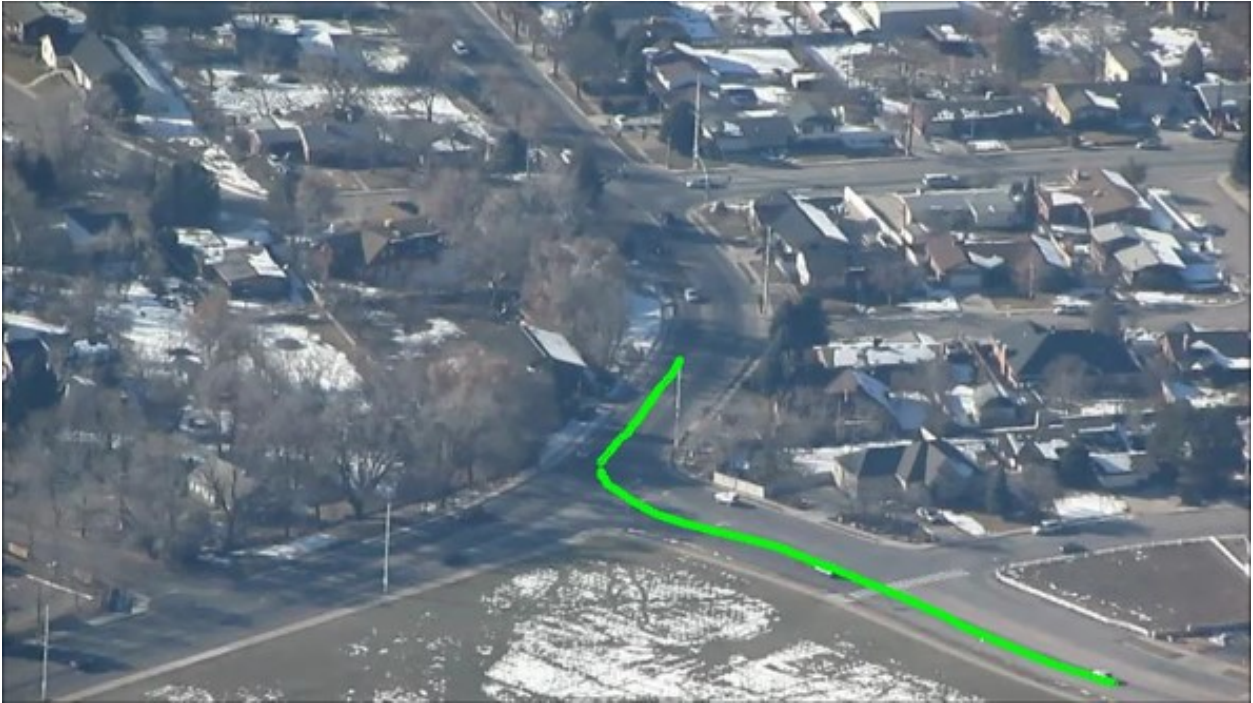
Figure 6.3: The R-RANSAC tracks associated with a car negotiating a moderate left hand turn. This version of R-RANSAC uses the nearly constant jerk motion model and completes the turn with a single track.
