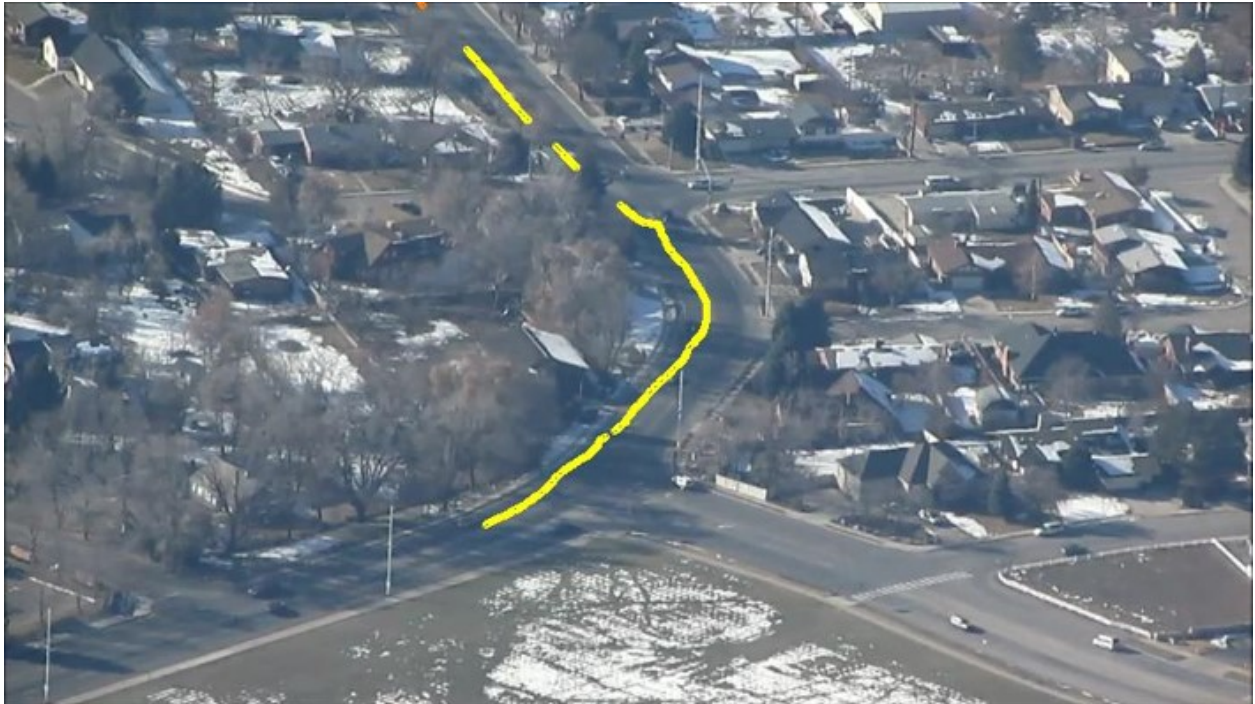
Figure 7.4: The two R-RANSAC tracks associated with one of the cars from the annotated section of the vehicle video. The first track is drawn in orange and appears on the top edge of the image.
