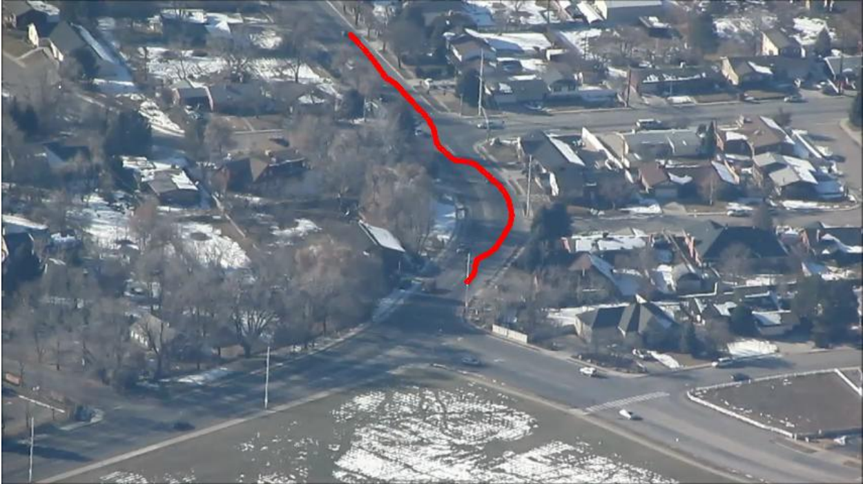
Figure 5.2: A single track produced by R-RANSAC with the nearly constant jerk model and probabilistic data association. The PDA filter provides robust tracking through the occluded intersection as evidenced by the single, continuous track.
