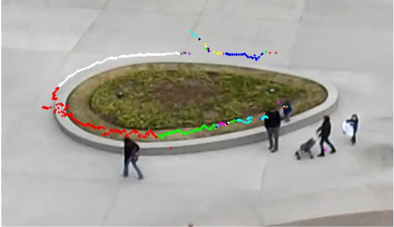
Figure 7.1: The GM-PHD tracks associated with one of the people from the annotated section of the pedestrian video.
