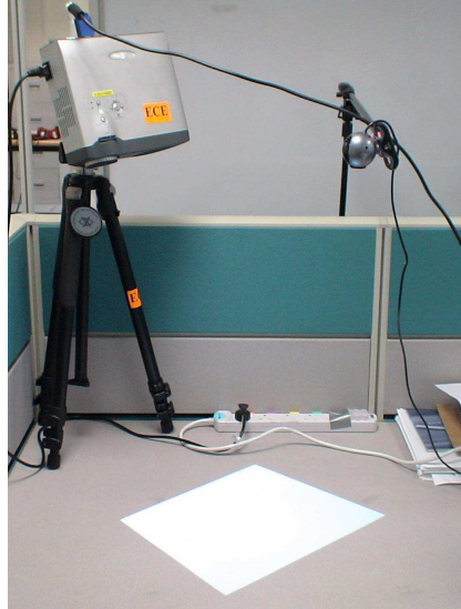
Fig. 1. System setup with the projector and the camera overlooking the tabletop. The projector and the camera can be casually and obliquely positioned, as long as the camera can see the projection area.
