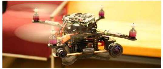
Fig. 1. The experimental platform with onboard computation (Intel Core 2 Duo 1.86 GHz processor) and sensing (right: primary fisheye camera, center: IMU, left: secondary camera).
