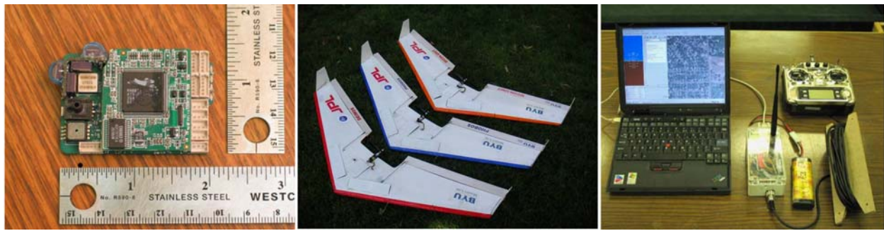
Fig. 6. (a) Kestrel autopilot. (b) Zagi airframes. (c) Ground station components.
