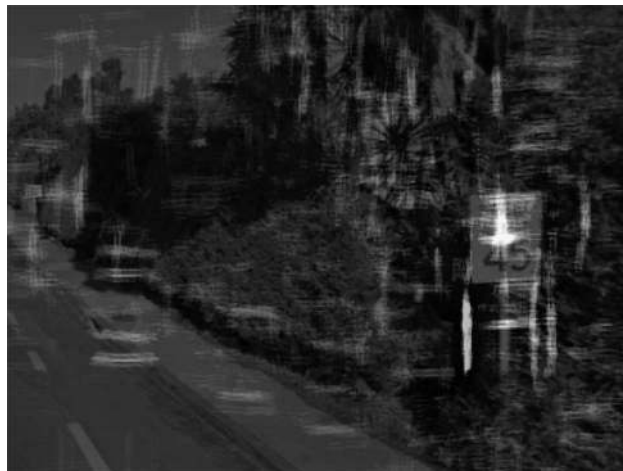
Fig. 11. Votes from a radial symmetry system superimposed on the original image. The brightest spot coincides with the center of the sign. This image is from a system developed in conjunction with this paper and is a radial symmetry voting algorithm extended to work for rectangles.
