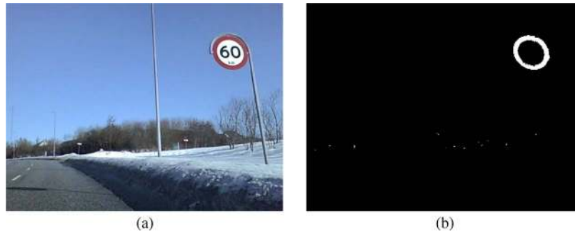
Fig. 8. Example of thresholding, looking for red hues. (a) Before thresholding. (b) After thresholding.
