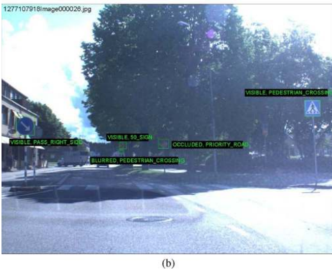
Fig. 6. Example sign images from (a) the GTSRB and (b) the STS Data set, with the sign bounding boxes superimposed.
