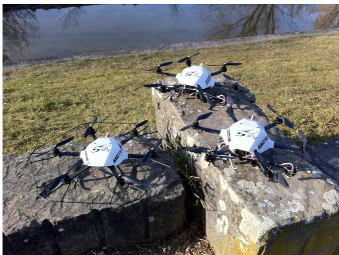
Fig. 1. The three SFLY hexacopters designed for inertial-visual navigation in GPS-denied environments.
