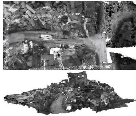
Fig. 19. Textured visualization of the 3D map of the firefighter area. (top and side view).
