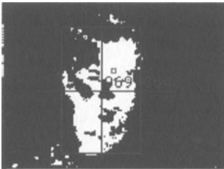
Figure 5 c. Thresholded skin probability with bounding box of connected components.
