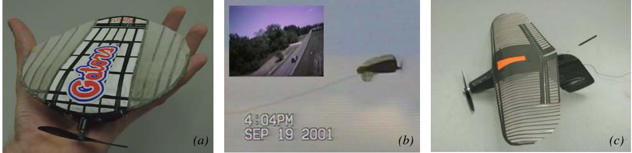
Fig. 1: (a) six-inch UF MAV, (b) six-inch UF MAV in flight with view through its on-board camera, and (c) 24-inch small UAV.
