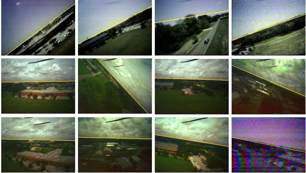
Fig. 2: Various horizon-detection examples under different lighting conditions (sunny and cloudy), and with varying degrees of video transmission noise. For each example, the yellow line indicates the algorithm’s horizon estimate.
