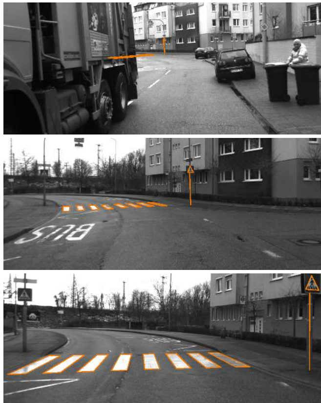
Fig. 1. The localization method allows to overlay infrastructural information of the map onto the current camera image after localizing the camera. The resulting augmented reality system demonstrates centimeter level accuracy of the proposed vision only localization method. A pedestrian crossing is reliably shown even when occluded by the truck. The “sensing distance” is unbound and does not increase computational load.
