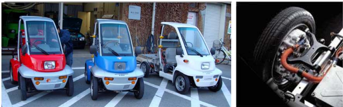
Fig.1. 3 Electric vehilces in Hori-Fujimoto laboratory and an in-wheel-motor.
