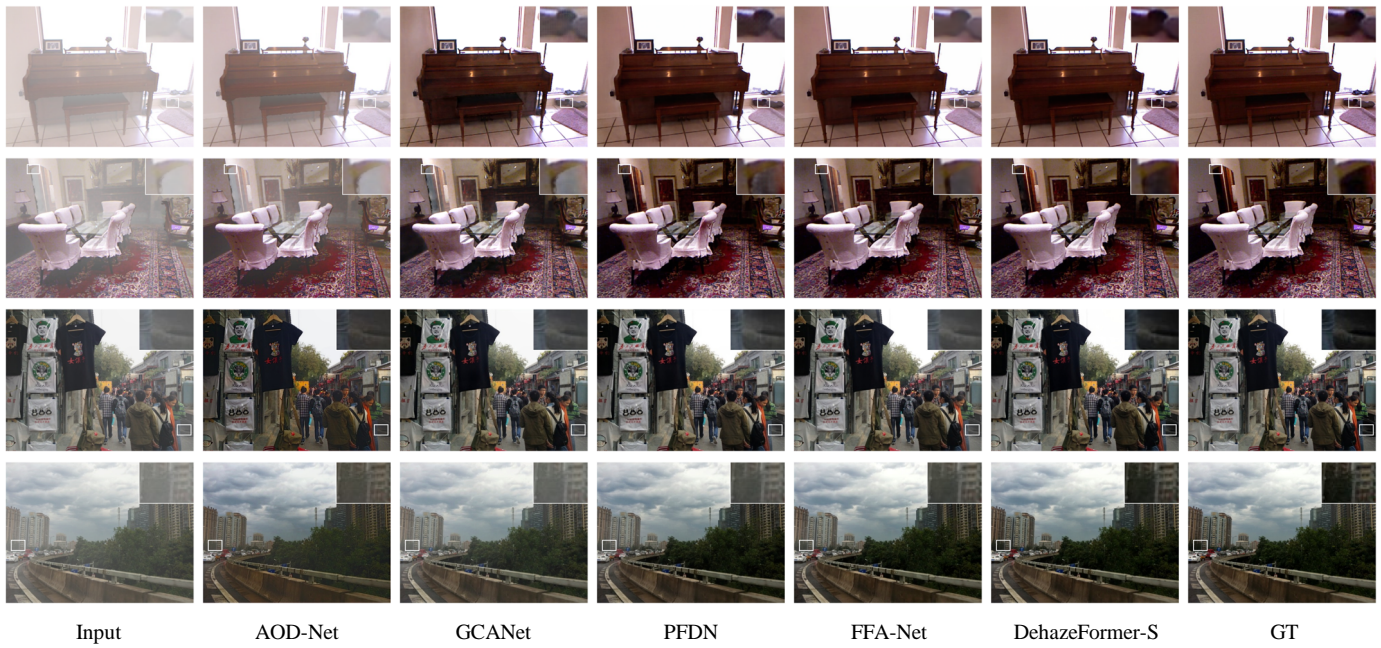
Fig. 7. Qualitative comparison of image dehazing methods on SOTS mix set, where the first two rows are indoor images, and the last two rows are the outdoor images. The first column is the hazy images and the last column is the corresponding ground truth.
