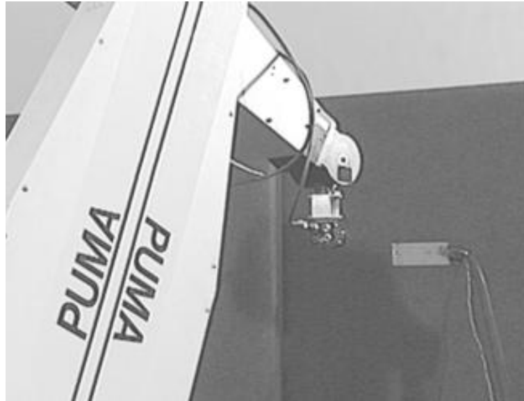
Figure 6.16: Photograph of square wave response test configuration. Small panel on the far wall contains the two LEDs.
