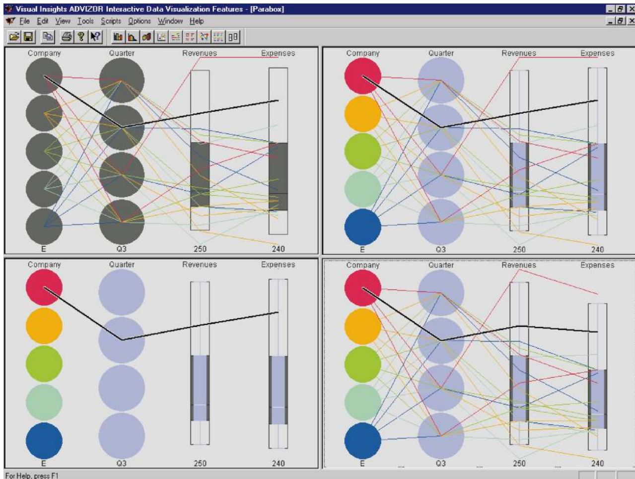
Fig. 5. ParaBox is a combination of Box plots and parallel coordinate plots for showing multidimensional data.
