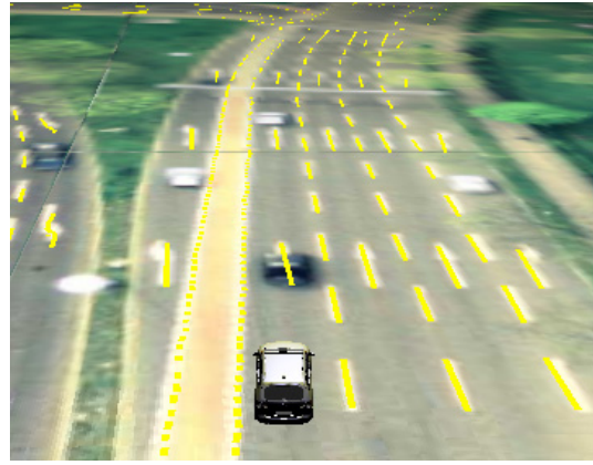
Fig. 10. Overlay of vehicle position, aerial image and lane markings (yellow) from the feature map.
