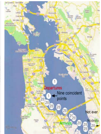
Fig. 2. The first and last positions where SFO controllers report useful visual information w/r to landing (RW 28) and departing aircraft RW 1).
