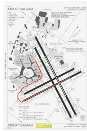
Fig. 1 SFO airport diagram showing typical movement paths for United Airlines, departures (dark/red), arrivals (light/green)
