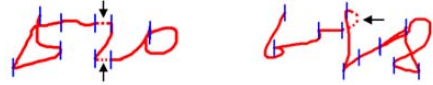
Fig. 4. Error examples when only “ dug ” is used. The strokes indicated by arrows are treated to be deleted strokes. However, they are parts of digit “2” and “9”, respectively. These strokes can be retained after “ dbg ” is used.
