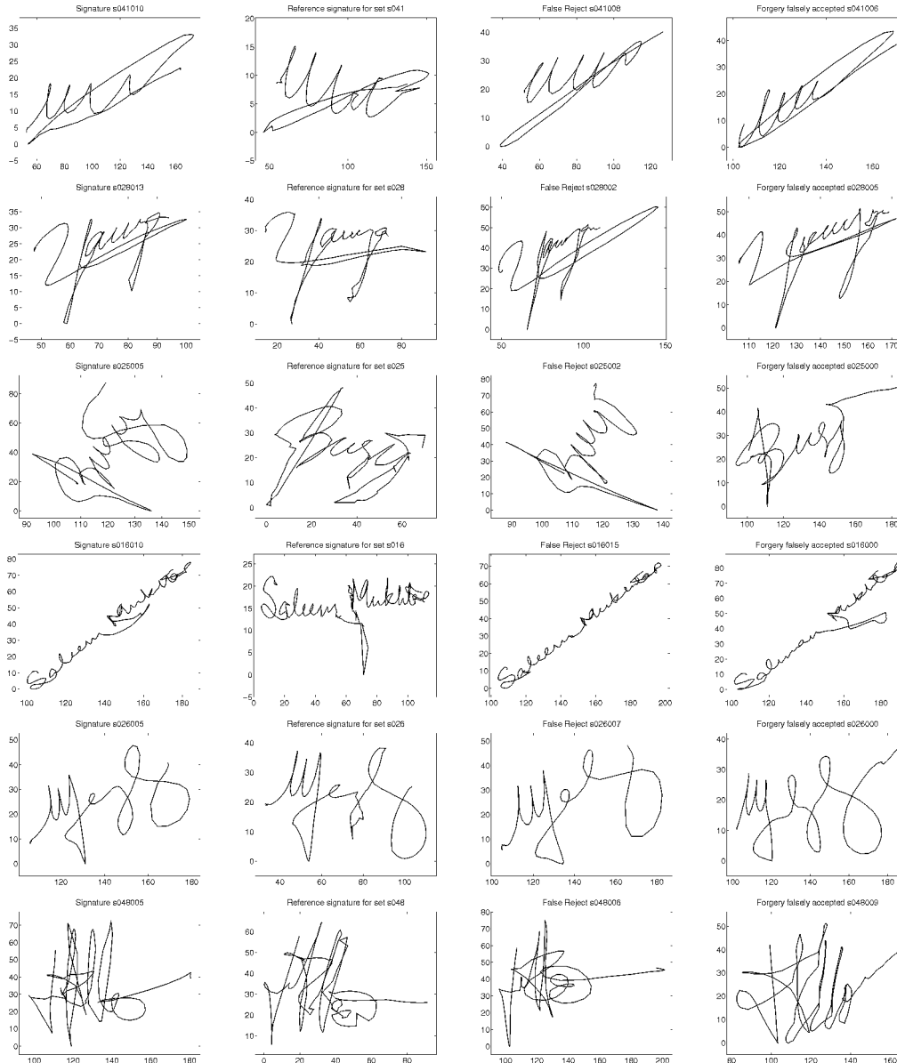
Fig. 19. Worst verification performance cases. Subjects with verification error rate greater than 5 percent. The three first subjects are from set 1 and the three last are from set 2. The plots show a visually-acquired signature, the corresponding prototype, a falsely rejected signature, and a falsely accepted skilled forgery. In the first four cases, high error rates correspond to signatures that are very simple and therefore easy to forge. The last two cases correspond to a subject (s026) whose signatures present a high degree of variability and to a subject (s048) for whom rotation normalization fails.
