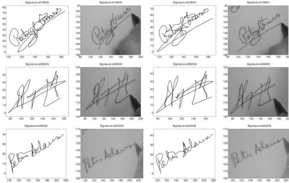
Fig. 5. Consistency of pen-up strokes. Examples of signatures acquired with the visual interface and corresponding images captured by the camera after finishing the acquisition. The images show the ink trace left on the paper, i.e., they display only the pen-down strokes of the signatures. The signature plots show the complete signing trajectories captured by the interface; these trajectories consists both of pen-down and pen-up strokes. The pen-up strokes of the signatures are as consistent as the pen-down ones; hence, we use the complete signing trajectory to perform signature verification and recognition.
