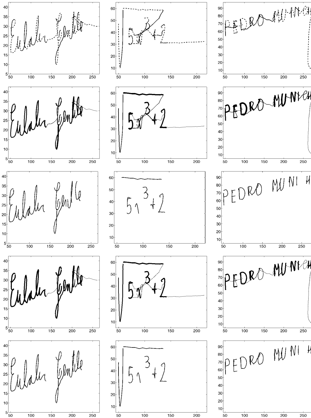
Fig. 14. Stroke classification results. The corresponding strokes for the sequences of Fig. 13 are shown on the first row. Successive strokes are plotted alternatively with solid or dashed lines. The figures of the second and third rows correspond to classification using the ink absence confidence measure; the figures of the fourth and fifth rows correspond to classification using HMM. The figures of the second and fourth row displays each stroke with a thickness that is proportional to the stroke confidence measure. The plots of the third and fifth rows show only the strokes classified as pen down in each case. The classification-based HMM seems to provide better results than the one based on the ink confidence measure.
