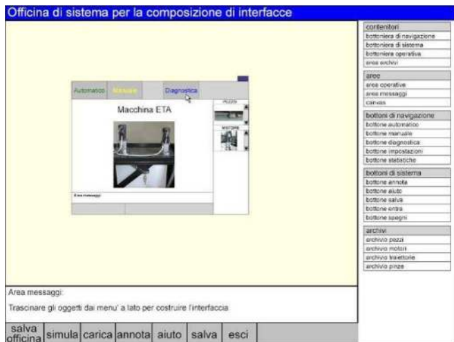
Fig. 15. Using W-Client system workshop, a d-expert is creating the application workshop shown in Fig. 12. The button “diagnostica” (diagnostic) is being located on the operative button panel.
