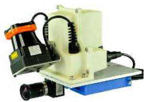
Fig. 8. Custom-built camera and lidar sensor. The camera is a uEye monochrome camera configured at 60Hz frame rate. The 3D lidar consists of a Hokuyo UTM-30LX laser scanner driven by a motor and an encoder that measures the rotation angle. The motor rotates back-and-forth at 180^\circ/s .
