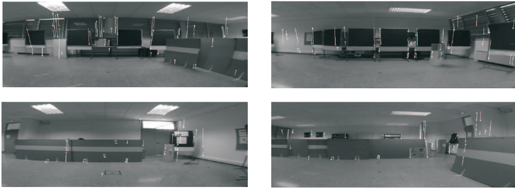
Figure 9: Reference images for the teaching phase with the extracted lines superimposed (after lens distortion correction). Each image is taken at a corner and in the direction of the next reference location.
