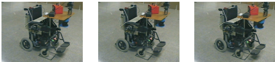
Figure 11: Position of the wheelchair after three, four and five rounds to the room. It can be observed that the differences are small enough.
