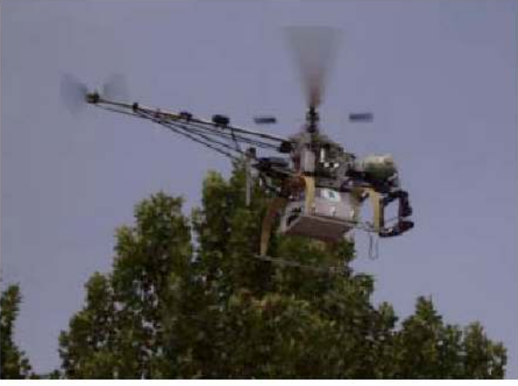
Fig. 1. UPM-COLIBRI I. HELICOPTER PLATFORM USED AS MAIN RESEARCH PLATFORM
