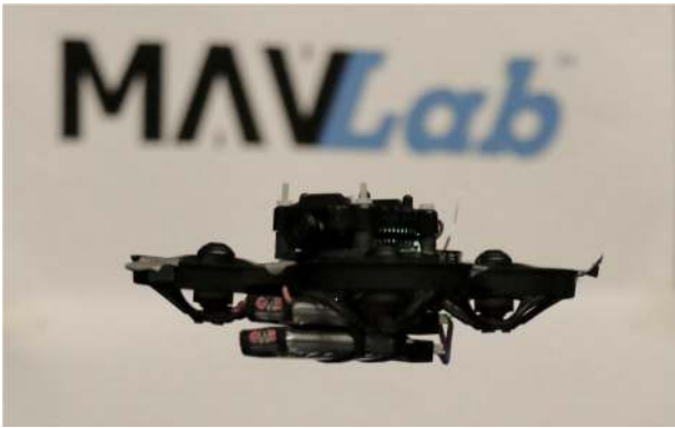
FIGURE 3 The flying platform. The Jevois is mounted on the Trashcan. The Trashcan provides power to the Jevois and they communicate with each other by the MAVLink protocol. The weight of the whole platform is only 72 g [Color figure can be viewed at wileyonlinelibrary.com ]
