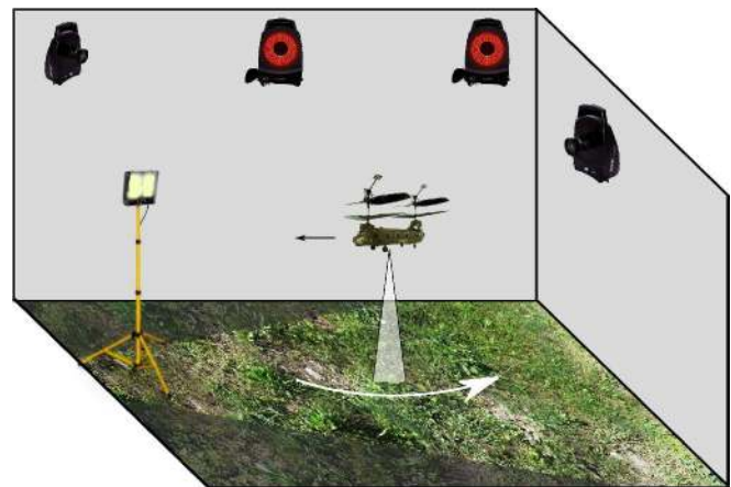
Fig. 5. The VICON-equipped free-flight facilities are composed of a ground covered with a natural pattern, a floodlight illuminating the scene in the visible domain and 6 VICON cameras to record the aircraft's motion. The floodlight was added because the background illuminance was initially only around 10lux in the VICON free-flying facilities.
