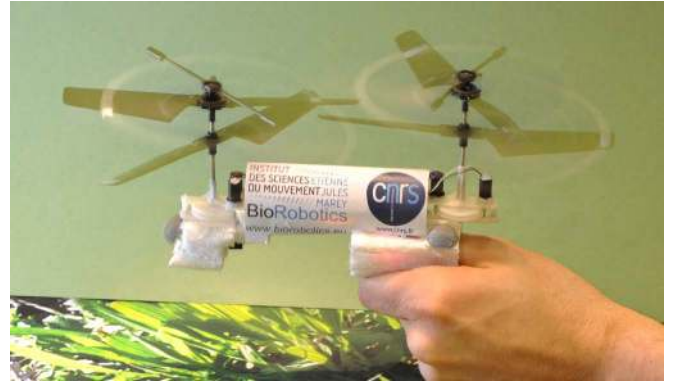
Fig. 2. TwinCoAx photograph showing the miniature free-flying helicopter equipped with a Bluetooth module and a programmable-gain visual motion sensor.
