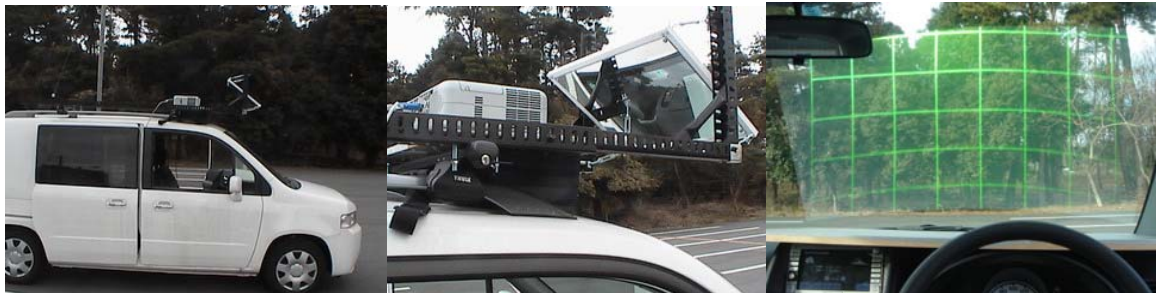
Figure 2 – External view of the WHUD system. The right picture shows the high luminance and wide display area of the WHUD.
